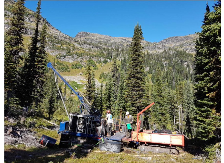
Tracked drill minimizes surface disturbance and tree-cutting
